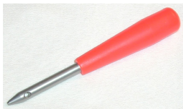
Figure 8-14 Use an eyelet punch to create holes in the center of each cross hair.
