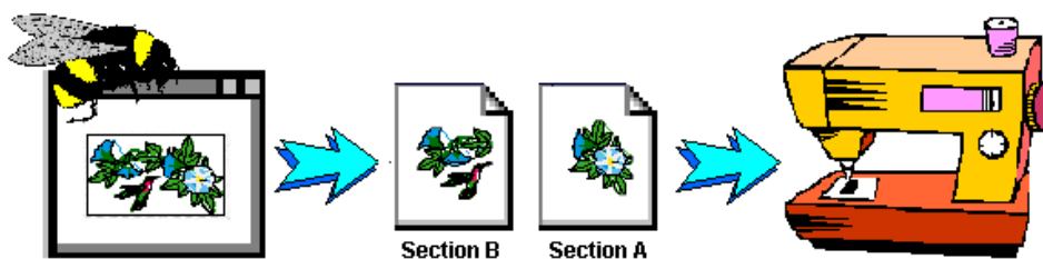
Figure 7-10 Design files are stitched on the machine one at a time in their assigned hoop positions to create the complete embroidery.
